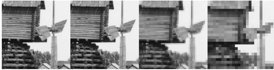
Fig. 4: Example of a four-level Laplacian pyramid for image 00859. Left-to-right: Bottom level of the pyramid (original image), Downsampled to \frac{1}{2} the resolution; Downsampled to \frac{1}{4} the resolution and Downsampled to \frac{1}{8} the resolution(resized to show detail)
